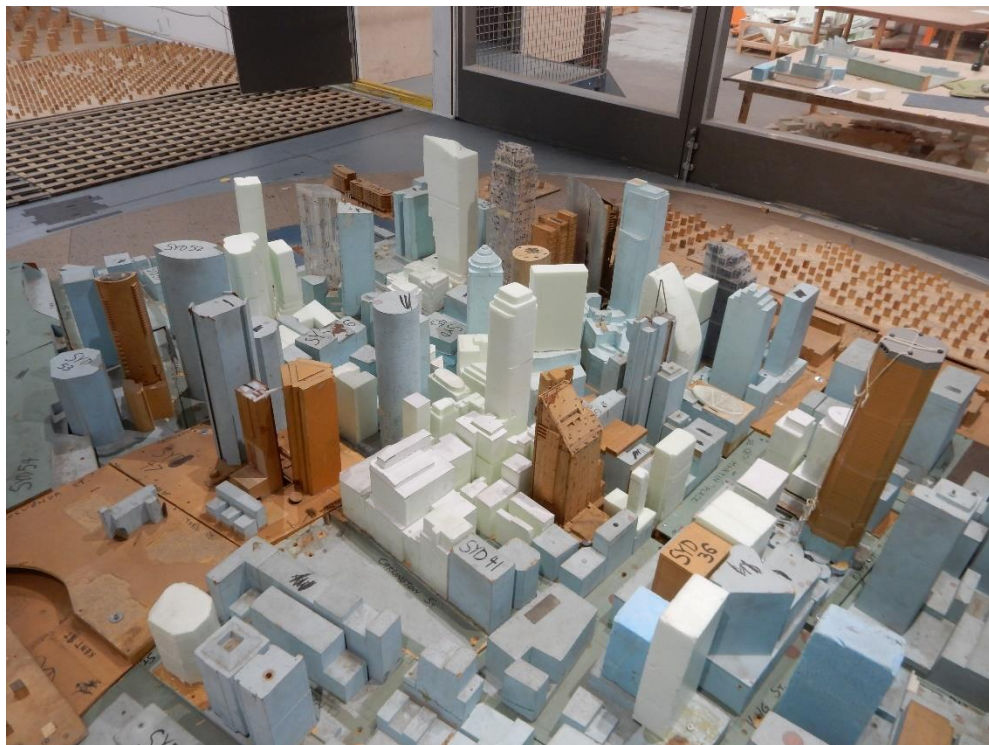
Figure 4 – View from the southwest of the 1/400 scale Proposed Configuration model of the 15-23 Hunter Street and 105-107 Pitt Street, Sydney in the wind tunnel.
